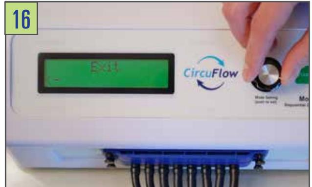
**17** Access the second parameter - Cycle Time, by turning the "SHUTTLE KNOB" to the right. Push the "SHUTTLE KNOB" to select Cycle Time.
