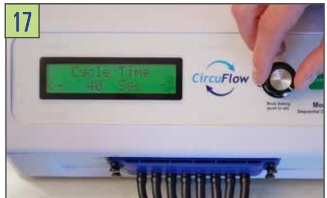
**18** Increase the Cycle Time by turning the "SHUTTLE KNOB" to the right, decrease time by turning to the left (cycle time can range from 20 – 240 seconds, increments of 1 second).
