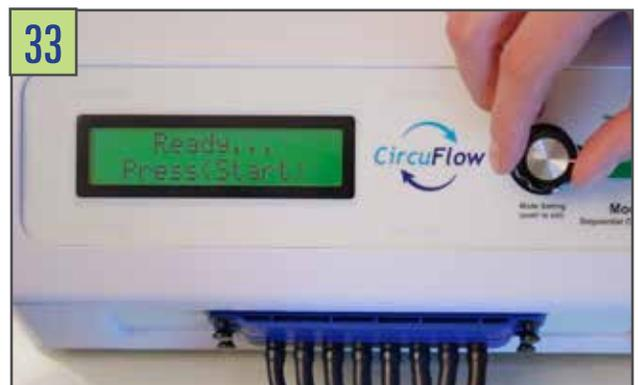
Please select "Unilateral" or "Bilateral" for one sleeve or two sleeve treatments by pressing down on the "SHUTTLE KNOB" to confirm. Continue to step 60.
