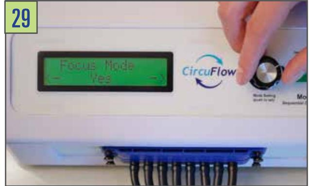
**30** Choose whether Focus Mode should be turned on or off. If it should be on, select which chambers to focus on, and what pressure to use, choosing between 40mmHg or 50mmHg.
