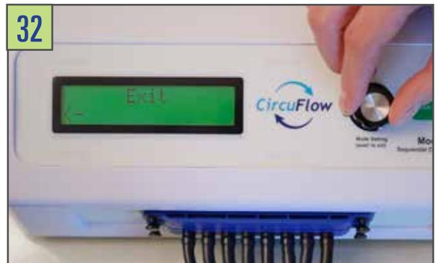
**32** To exit and complete Pressure Mode setup, turn the "SHUTTLE KNOB" to the right. Push to select to Exit.
